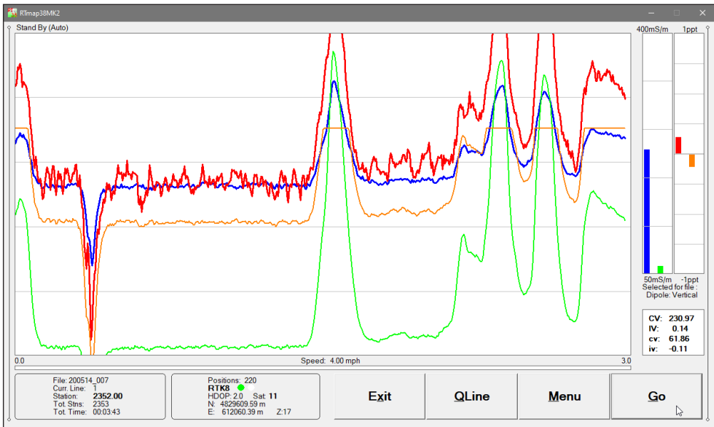
Figure 8.31: RTmap38MK2 in Stand By mode and Profile display mode
